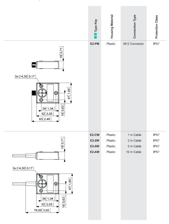
$All\ dimension\ in\ mm\ [inch];\ Al:\ Aluminum;\ 303:\ Stainless\ Steel\ V2A\ (1.4305,\ 303);\ 316\ L:\ Stainless\ Steel\ V4A\ (1.4404,\ 316\ L)$
