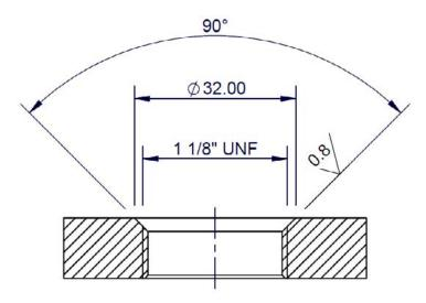
Fit the O-ring above the male thread on the sensor. Ensure the O-ring is centred and sits within the chamfer; tighten the sensor using a adjustable spanner until the sensor face is flush with the top of the tank and a torque of 50 Nm is achieved.
