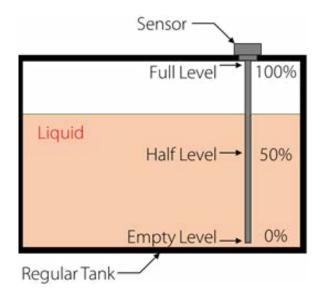
The sensor is supplied so that it reports the level in a linear path as the level rises. However, this will not be suitable for an irregular shaped tank, such as that shown below.
