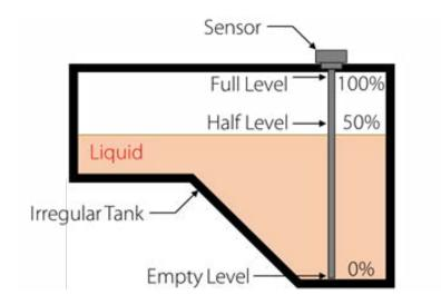
In this situation, 50% of the tank volume is not half way up the probe. To correct for this tank profiling can be used. This can be done in the GSlevel software and is covered in detail in the GSlevel User Manual.
