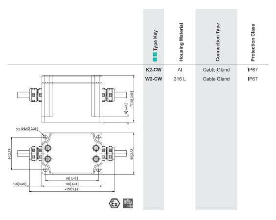
All dimension in mm [inch]; Al: Aluminum; 303: Stainless Steel V2A (1.4305, 303); 316 L: Stainless Steel V4A (1.4404, 316 L)
