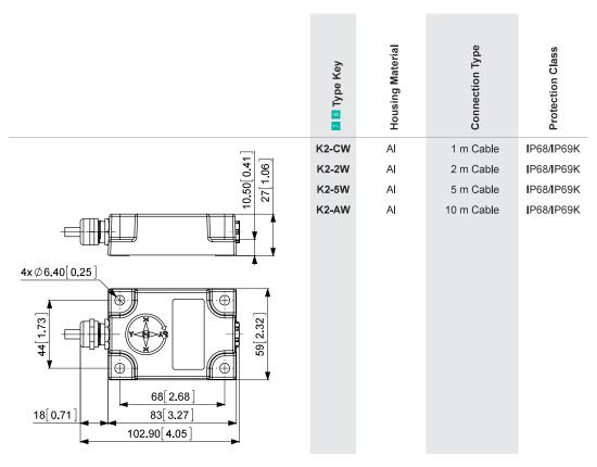
All dimension in mm [inch]; Al: Aluminum; 303: Stainless Steel V2A (1.4305, 303); 316 L: Stainless Steel V4A (1.4404, 316 L)
