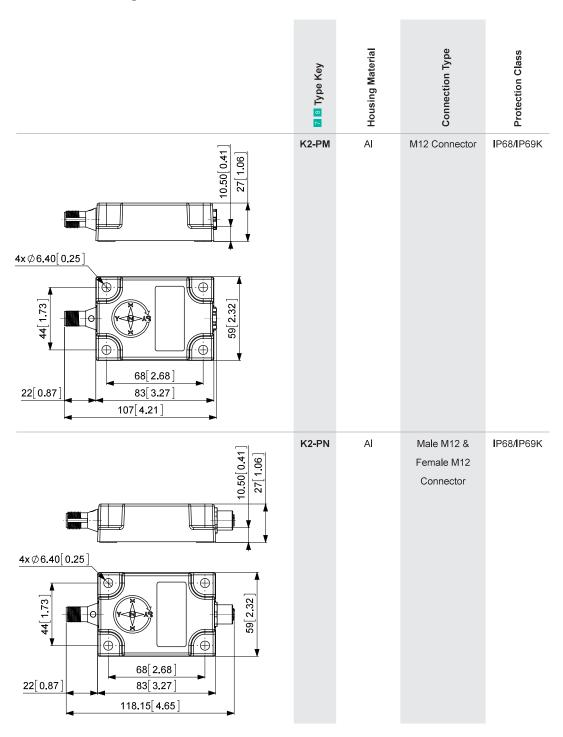
All dimension in mm [inch]; Al: Aluminum; 303: Stainless Steel V2A (1.4305, 303); 316 L: Stainless Steel V4A (1.4404, 316 L)
