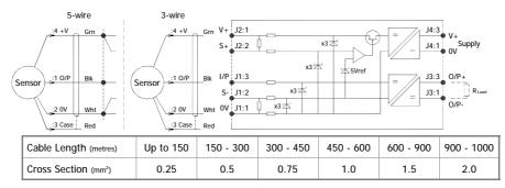
The table above shows recommended conductor sizes with respect to cable length for both three and five wire connections, based on copper conductors. Three wire connections will introduce a gain reduction of 5% and a  $\pm$ 1% temperature dependence of gain over the range -40°C to +80°C for the cable temperature. (i.e. about –150 ppm/°C for the maximum lengths shown and less pro rata for shorter lengths.)
