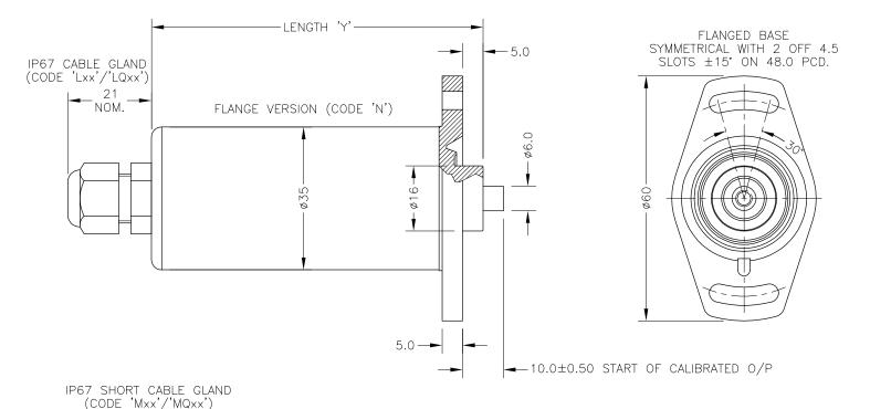
GAIN AND OFFSET ADJUSTMENTS SEALED (CODE 'Y')
