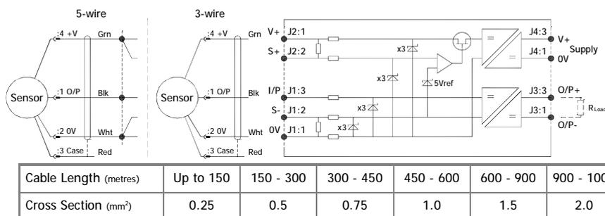
The table above shows recommended conductor sizes with respect to cable length for both three and five wire connections, based on copper conductors. Three wire connections will introduce a gain reduction of 5% and a ±1% temperature dependence of gain over the range -40°C to +80°C for the cable temperature. (i.e. about -150 ppm/°C for the maximum lengths shown and less pro rata for shorter lengths.)
