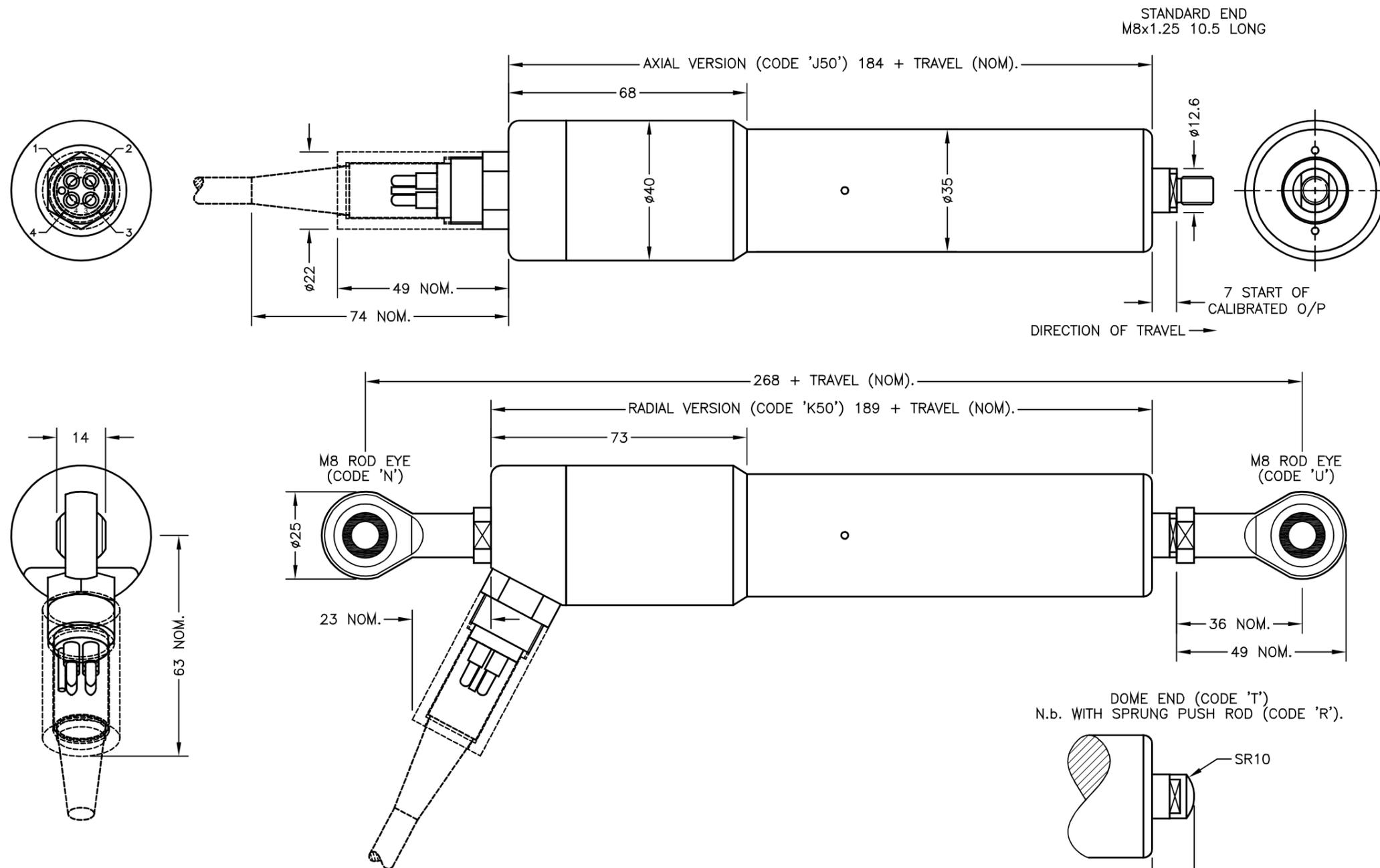
MAXIMUM WORKING DEPTH: 3500 METRES 350 BAR. WHERE THE FREE END OF THE CABLE IS TO BE TERMINATED IN A SUBMERGED POSITION, ADEQUATE SEALING MUST BE PROVIDED TO PROTECT CONNECTIONS.
