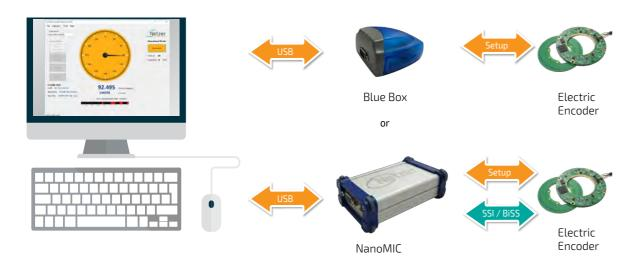
Connect Netzer encoder to the converter, connect the converter to the computer and run the Electric Encoder Explorer Software Tool
