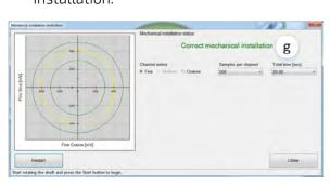
(h) If the SW indicates "Incorrect Mechanical Installation," correct the mechanical position of the rotor, as presented in paragraph 3.3 - "Rotor Relative Position."
