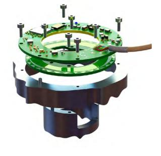
Encoder stator / Rotor relative position For proper performance the air gap should be 0.6 mm +/- 0.1mm
