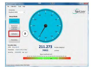
(b) Start the data acquisition while rotating the shaft.
