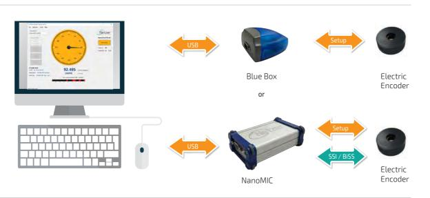
Connect Netzer encoder to the converter, connect the converter to the computer and run the Electric Encoder Explorer Software Tool
