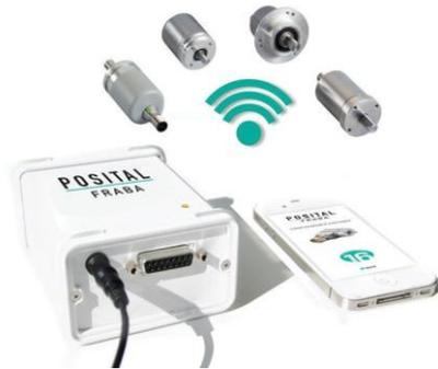
Thank you for purchasing our UBIFAST Configuration Tool. The UBIFAST Configuration Tool is used to configure the parameters of POSITAL's IXARC programmable encoders through a simple browser based programming interface. Please read this leaflet thoroughly and carefully before installation and using the device.
